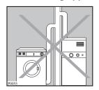
Note that to avoid condensation problems, it is essential that the dryer be fitted with the flexible hose to carry its "exhaust" at least beyond the kitchen units; preferable outside the kitchen.
